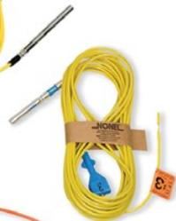
NONEL SL (short lead) detonators are designed to be used with low energy detonating cord downlines. When used in a slider configuration, they provide independent deck initiation from a single downline. Each unit consists of a precise millisecond delay detonator assembled to a 30 inch (76 cm) length of sealed orange shock tube with a looped end.
