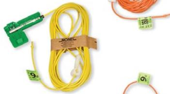
NONEL MS Connectors are used with detonating cord initiated blasts to provide millisecond delay timing between holes and rows. This bi-directional trunkline connector consists of an 18-inch (46 cm) length of shock tube with millisecond detonators of the same delay, inside color-coded connector blocks, on each end.
