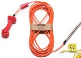
NONEL EZTL® trunkline delay detonators feature precise millisecond delay timing and hardware suitable for use as trunklines in open pit and underground mining, as well as quarrying and construction. These detonators consist of a length of yellow shock tube attached to a low strength millisecond delay detonator housed in a plastic EZ Connector block on one end and sealed with a plastic J-hook attached to the other end.
